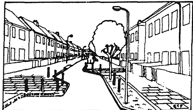
FIG 7: CHICANE DESIGN SHOWING 2 STREETS WITH + WITHOUT CHICANES
