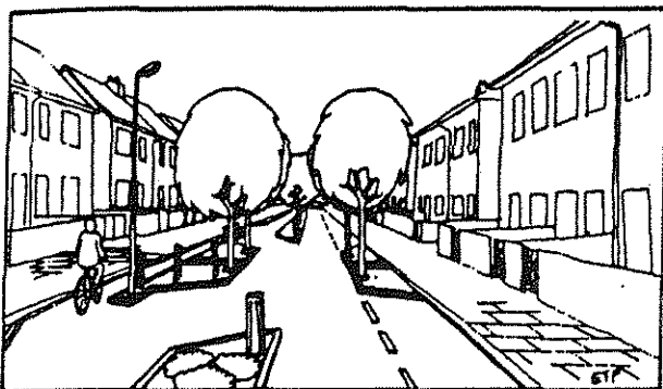
FIG 7: CHICANE DESIGN SHOWING 2 STREETS WITH + WITHOUT CHICANES
